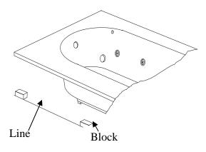
7. For final skirt installation and to allow for removal if necessary in the future, adhere skirt to wooden back support blocks with silicone or other removable adhesive. Place a straight board against front bottom of skirt to hold it firmly in place while the adhesive cures.
